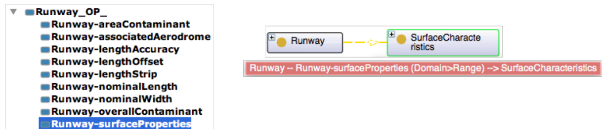
Figure 17. A UML aggregation relationship is transformed to an OWL Object Property (with domain Runway and range SurfaceCharacteristics)
