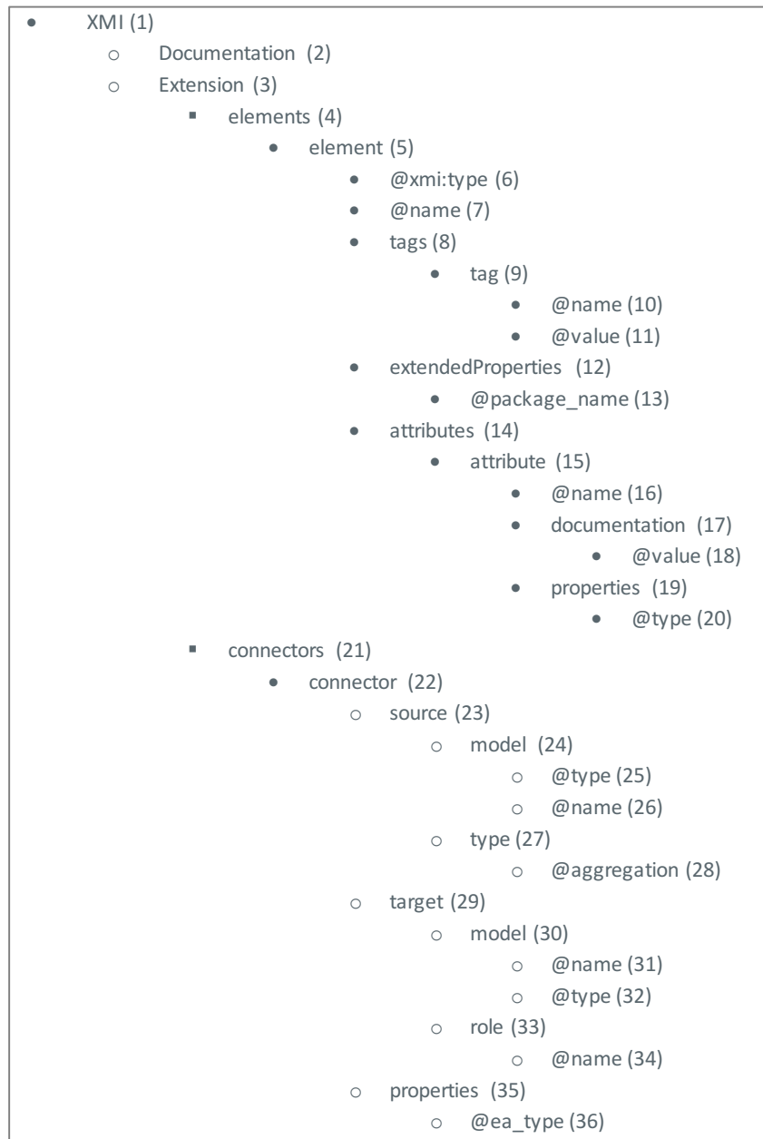
Figure 7. Structure of the XMI generated from the AIRM UML Model.
